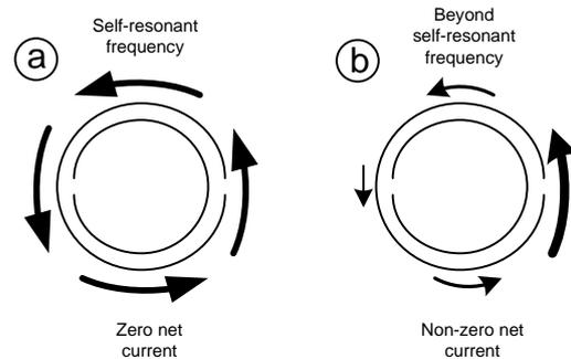
Fig. 4 Comparison between the current distribution on the SRR at the resonant frequency (a) and beyond the resonant frequency (b).
