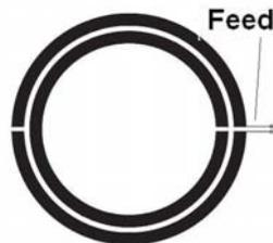
Fig. 3 SRR feed through a small gap in one of the two rings.
