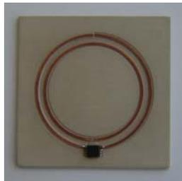
**Fig. 6** Prototype of the SRR tag antenna.
