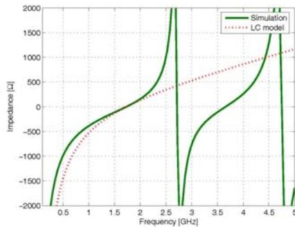
**Fig. 5** Comparison between LC model and simulation. SRR has parameters:  $r_o=8.75\text{ mm}$ ,  $c=1\text{ mm}$  and  $d=0.5\text{ mm}$ . LC model has parameters:  $L=42.11\text{ nH}$  and  $C=0.201\text{ pF}$ .
