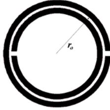
**Fig. 1** Structure and relevant dimensions of the SRR.
