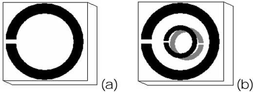
**Fig. 3** Structure of the small loop (a) and the small loop with the BC-SRR core (b).
