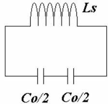
**Fig. 2** Equivalent circuit model of the SRR.
