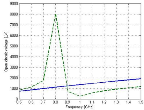
**Fig. 4** Comparison between the open circuit voltage of a small loop and a small loop with SRR core.
